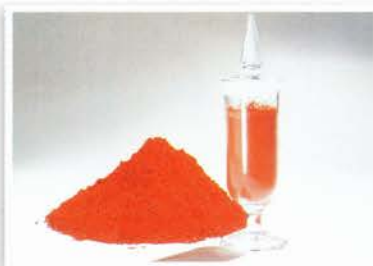
Cuprous Oxide Used as Antifoulant for Ship-Bottom Paints
